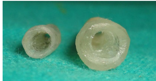
Fig. 9 Final hollowed nasal stents
