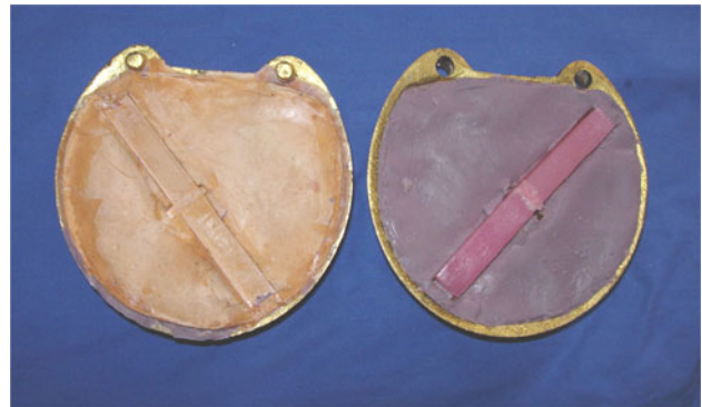
Fig. 4 Liner placed inbetween the two resin blocks
