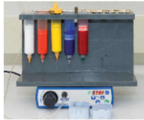
Fig. 1 EFD ® , Engineered Fluid Dispenser, Performus ™ II (source: http://www.efd-inc.com ), adapted to several of the syringes with pigment pastes
