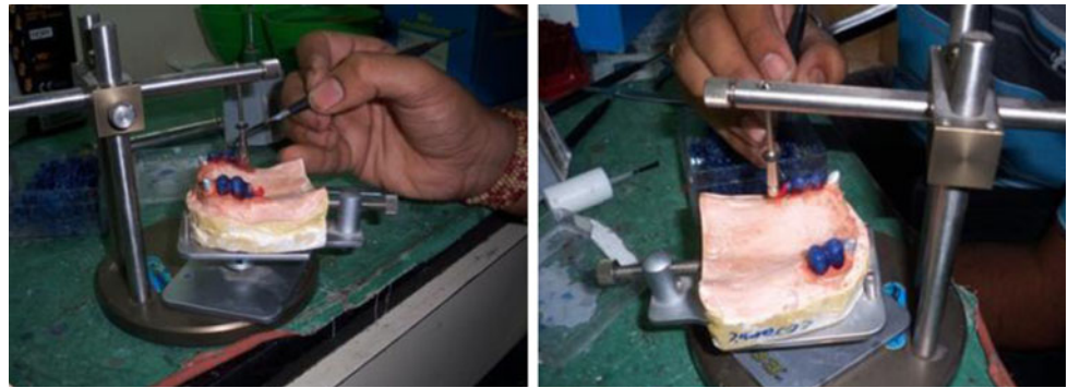
Fig. 7 Attaching the stud attachment to the wax pattern with the help of parallelometer
