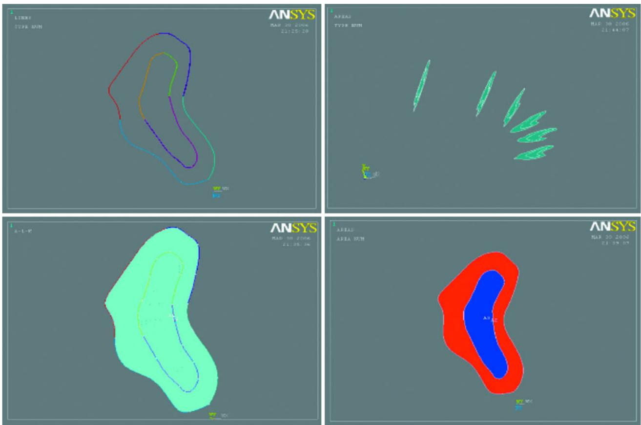
**Fig. 2** Line geometry, surface geometry and solid geometry of cortical bone
