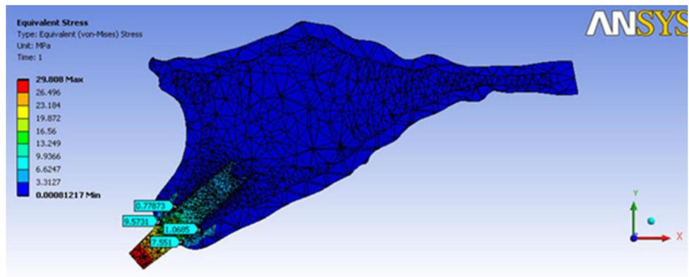
**Fig. 3** Von Mises stress around implant with straight abutment in D3 bone
