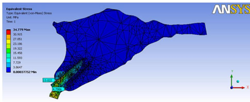
**Fig. 6** Von Mises stress around implant with angled abutment in D2 bone
