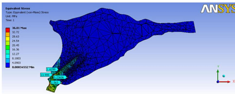
**Fig. 7** Von Mises stress around implant with angled abutment in D3 bone
