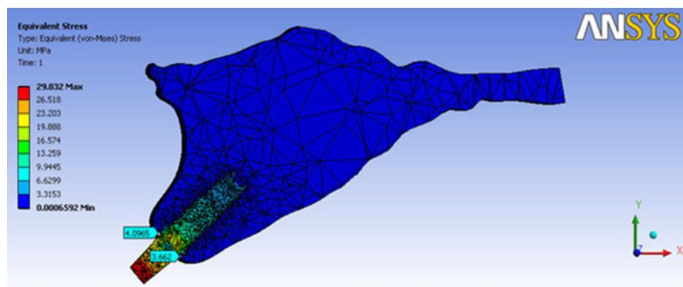
The implant abutment complex was modeled as a one piece structure and the crown restoration was omitted because the primary aim of the study was to analyze the stress distribution around the implant and not to study the stress distribution at the implant–abutment or the abutment–prosthesis interfaces [19].
