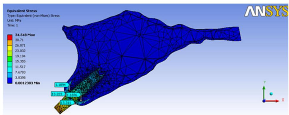
**Fig. 4** Von Mises stress around implant with straight abutment in D4 bone
