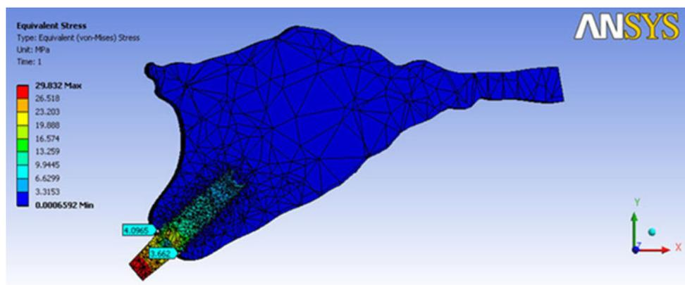
**Fig. 2** Von Mises stress around implant with straight abutment in D2 bone
