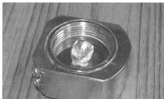
Fig. 5. Gold Coating done over fractured PFM specimen
