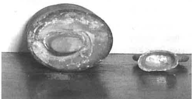
Fig V: Adhesive failure - cement on tooth
