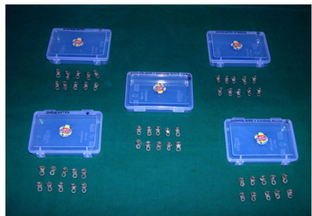
Fig. 2 Samples with surface treatment (10 each of Group U, S, SK, UD and UDK)
