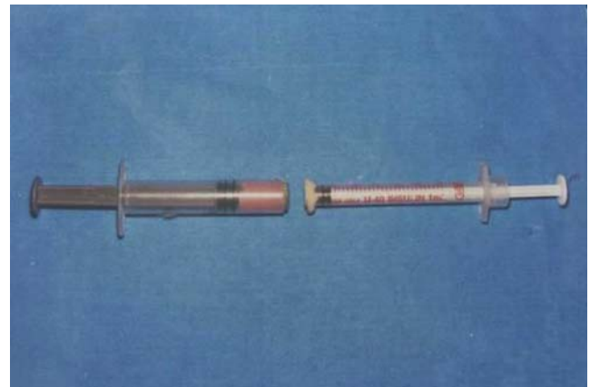
Fig. 4 Separated specimen after adhesive strength testing
