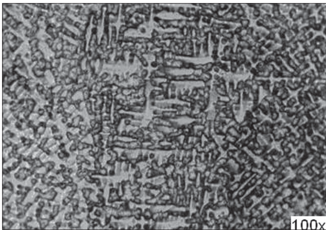
Figure 6: Microstructure after the 2 nd cycle of heat treatment (650°C)
