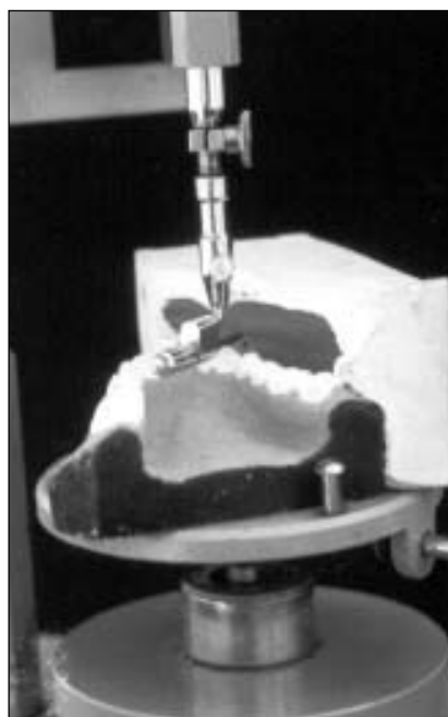
Figure 5: Procedure for marking the occlusal plane with a custom-made marking accessory
